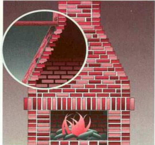
This funnel shape is usually formed by Corbelling brick or block. **Corbelling** is a method of laying bricks like steps to achieve a desired shape.
